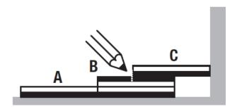
Now indicate on Tile B where you have to cut. Finally, install the cut Tile B in the space between the wall and Tile A.
